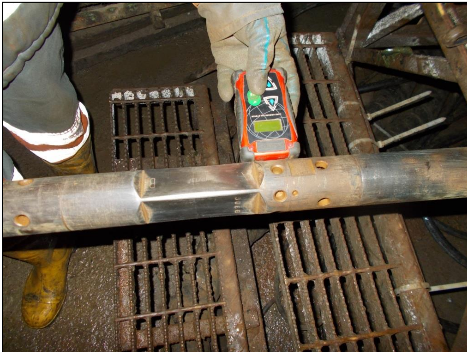
Figure 10-3: Process of core orientation at underground drill site by a driller using Orifinder controller (DPMC, 2015)
