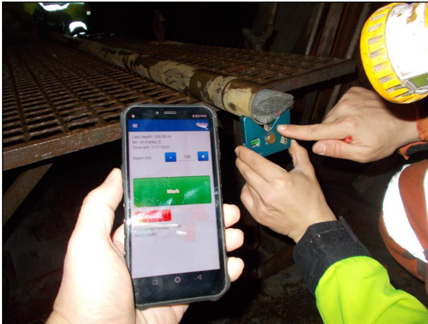
Figure 10-4: Process of core orientation at underground drill site by a driller using DeviCore instrument (DPMC, 2021)
