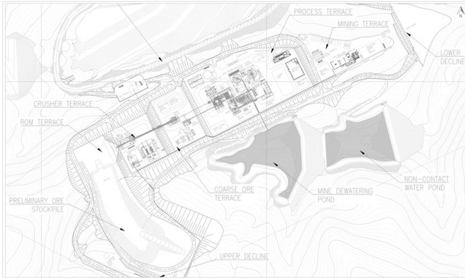
Figure 18.2 – Process Plant Layout
