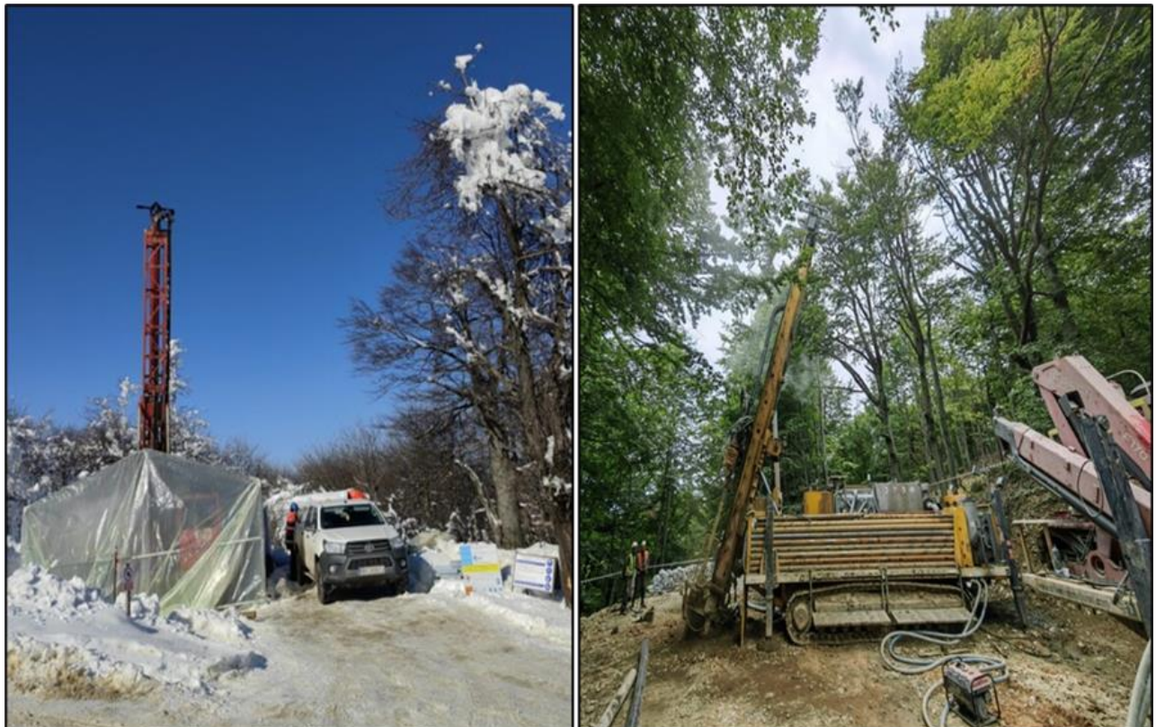
Figure 10-1: Diamond drill rig (left) and a RC drill rig (Right) at Čoka Rakita Source: DPM, 2023
