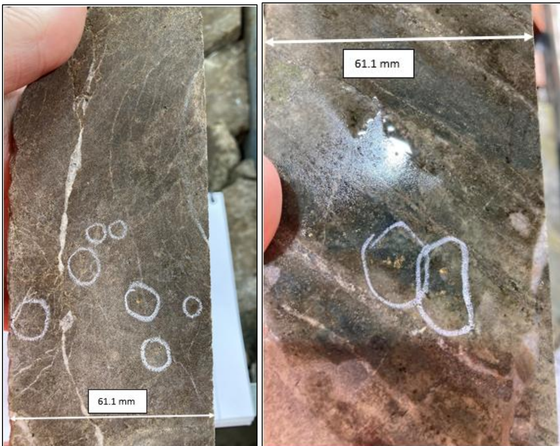
Figure 12-4: Visible gold seen in core in drillhole RIDD008 Source: CSA Global, 2023
