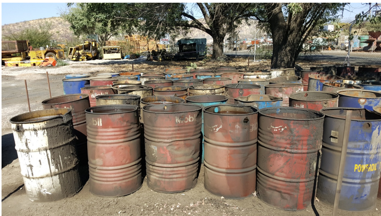
Plate: Uncovered and damaged drums with waste oil and sludges stored in an unbunded area
