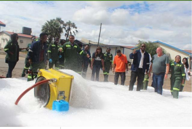
The Dundee Precious Metals Tsumeb Emergency Response Department showcase the portable foam generator. It is designed to expand foam solution into millions of tiny stable bubbles specially engineered to extinguish chemical fires The Dundee Precious Metals Golden Rules are a series of procedures and instructions that govern activities in the daily work routine.
