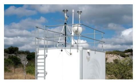
Sulphur dioxide (SO<sub>2</sub>), particulate dust (PM10) and arsenic (As) monitoring station – Tsumeb.
